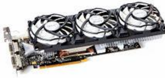
A 3-fan heat sink mounted on a graphics card
