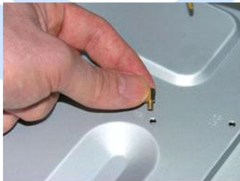
Figure 9: Screw Brass Standoffs Into the Motherboard
