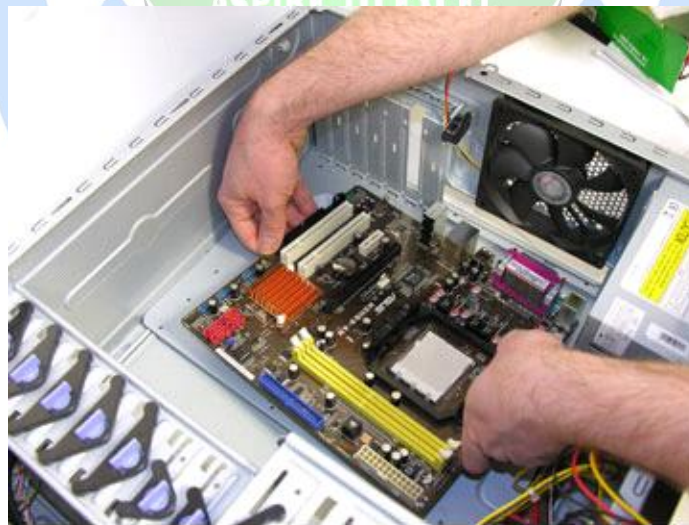
Figure 11: Mount the Motherboard
