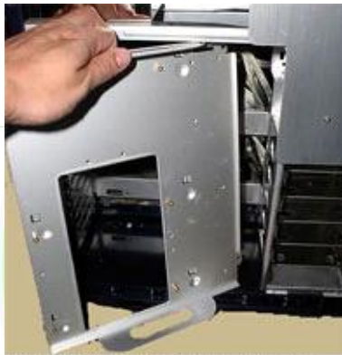
Figure 8: Remove Motherboard Tray
