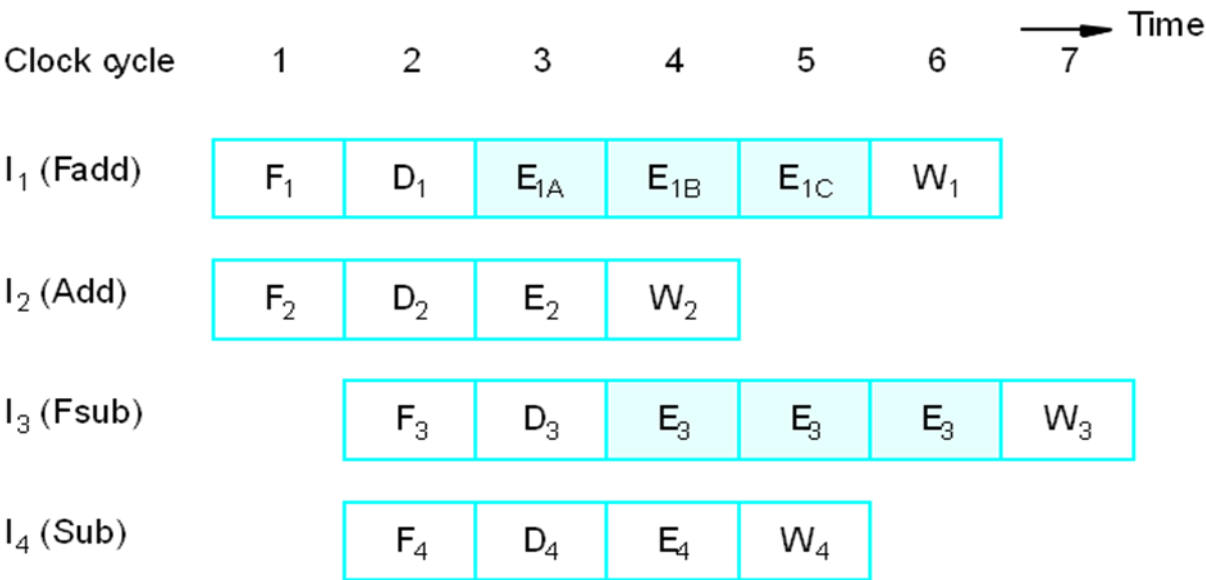
Fig.An example of instruction execution flow in the processor assuming no hazards are encountered.
